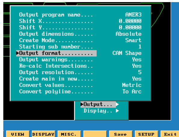
Figure 17-4, DXF Output format, CAN Shape Pop-up Menu Illustration
